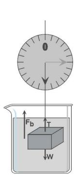
We can use a spring scale to determine  $F_{net}$  and calculate  $F_B$ :
